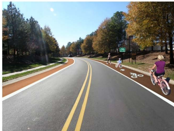
Proposed bike lane treatment along Brandon Oaks Pkwy
